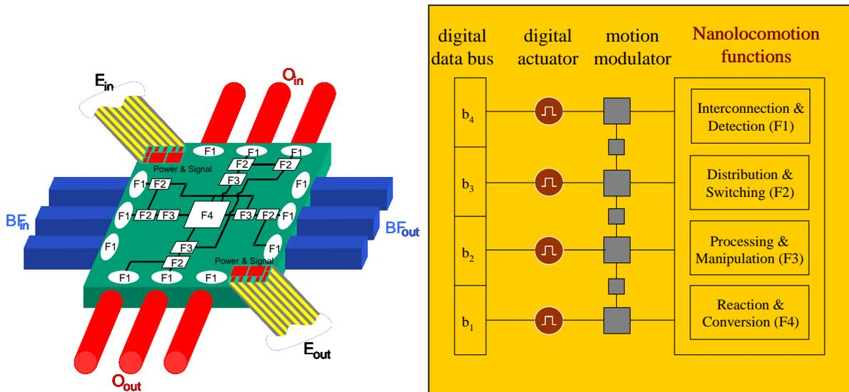
(a) Physical model in the form of digital muscle chip. (b) Functional decomposition of components.
