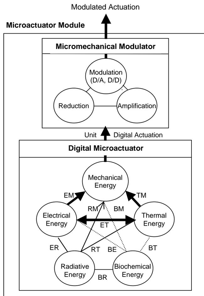
Fig.3 Energy transduction and manipulation for nanolocomotion.
